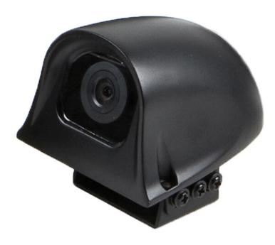
The RVS-775-ADH is a commercial grade analog HD side camera. This backup camera was designed solely for our mobile DVR's and have a HD resolution of 1280 (H)  $\times$  720 (V). It boasts 120° viewing angle and is completely waterproof with an IP69K rating.
