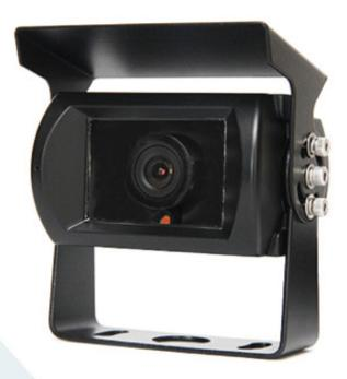
The RVS-770-ADH is a commercial grade analog HD backup camera. This backup camera was designed solely for our mobile DVR's and have a HD resolution of 1280 (H)  $\times$  720 (V). It boasts 120° viewing angle and a built in microphone which enables you to hear what is behind you. The backup camera is completely weatherproof with an IP69K rating, and comes with a full year warranty.
