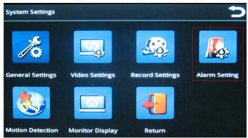
The Alarm Settings menu enables you to set alarm properties for each of the six trigger channels, which are selectable from the channel pull-down menu.
