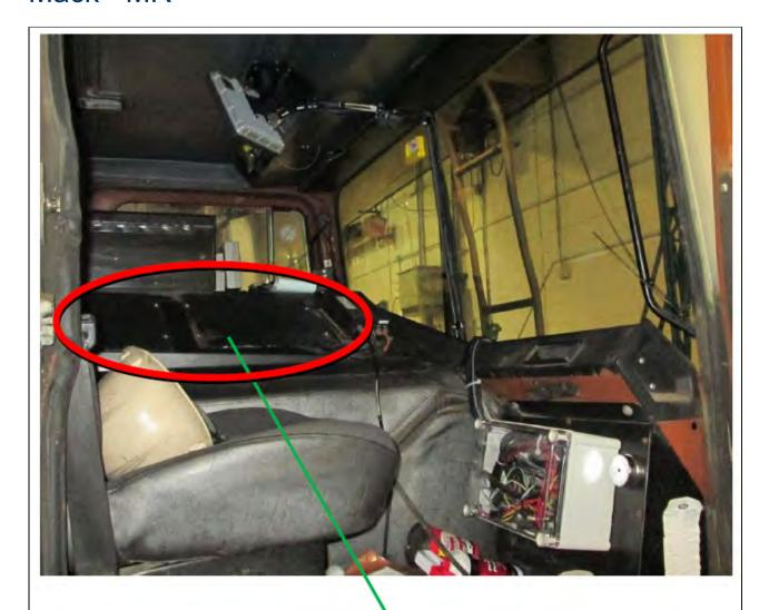
12v, Ground, Reverse and Brake (stop lamp) are located behind these 2 access panels along a labelled busbar similar to the Mack MRU
