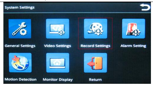
The Record Settings menu enables you to set recording properties for each of the six channels, which are selectable from the channel pull-down menu.
