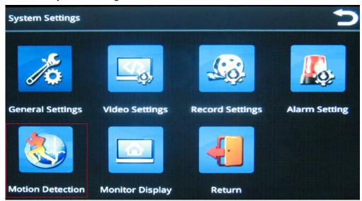
The Motion Detection menu enables you to set motion detection properties for each of the six channels, which are selectable from the channel pull-down menu.
