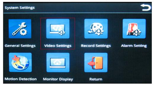
The Video Settings menu enables you to specify video properties for each of the six channels, which are selectable from the channel pull-down menu.
