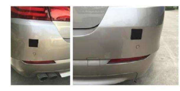
Step 3: Remove the rear bumper to clean the suface for sensors.
