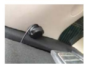
Step 8: Tuck the wires neatly to hide and prevent wire pinch.
