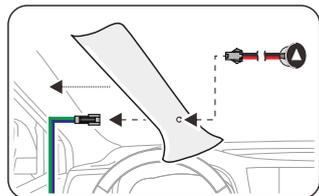
Thread the LED alert terminal and wire through the fresh mounting hole and connect the alert cable. Snap the LED alert into the mounting hole. Then install the cover back to the A-pillar.
