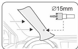
Take the A-pillar trim cover off and locate a spot which is close to the sightline to the side mirror. Drill the LED alert mounting hole with the included 15mm hole saw in counter-clockwise mode.
