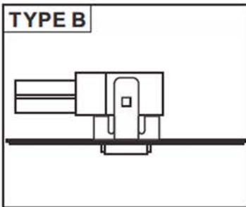
① locate the spot for mounting hole at the side of the rear bumper. Then drill with the included 16.5mm hole saw in counter-clockwise mode. ② Snap the radar sensor into the mounting bracket and attach the double-side 3M sticker.
