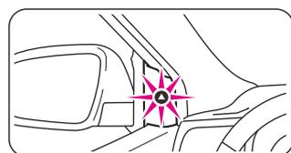
LED alert can be drilled on the triangular panels on the front door if a sufficient space for mounting is available.
