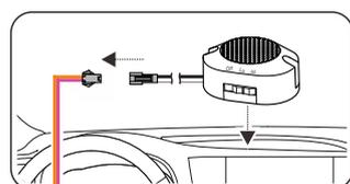
Put the buzzer on the dash and fasten with included double-sided sticker, connect the wires to the control module.
