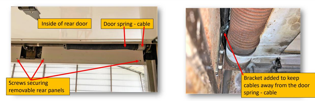
When running the camera and sensor cables across the back of the cargo box, route behind removable panels if possible. **Note:** If the RVS cables are in contact with the door cable, they could be rubbed through. These doors are opened and closed many times and it may be necessary to add a bracket of some kind to keep the RVS cables away from the door spring cable.
