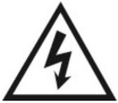
This symbol is intended to alert the user to the presence of uninsulated "dangerous voltage" within the product's enclosure that may be of sufficient magnitude to constitute risk of electric shock to persons.
